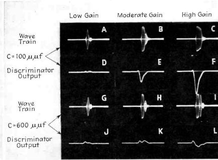
Fig. 2—Oscillograms of noise wave train and output of discriminator showing detuning due to grid current at higher amplitudes
