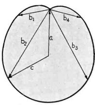
Fig. 6—Vector diagram corresponding to Fig. 5. Signal-to-noise ratio is 0.5. Relative phase is 180 degrees at peak of noise
